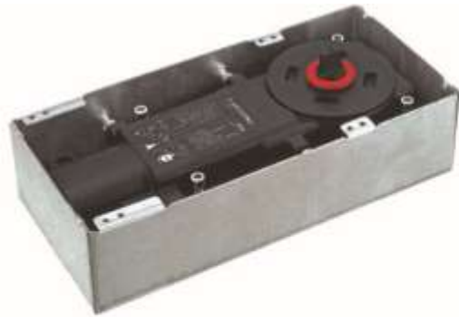
1 section adjust 150° -25° closing speed 2 section adjust 25° -0° closing speed
